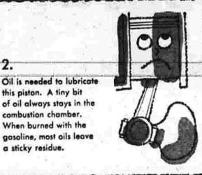
particles are formed by the gasoline explosion. These particles should escape through the exhaust. But the sticky oil residue traps and "glues" some of them to
